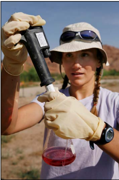
Photo: Liz Glowiak, Pro2Serve hydrogeologist on the Technical Assistance Contract team, measures the alkalinity of a ground water sample.
